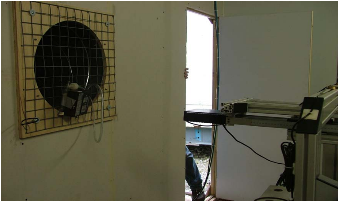
Figure 15. Impinger/Filter Sampler on Extract Fan – Initial set-up
