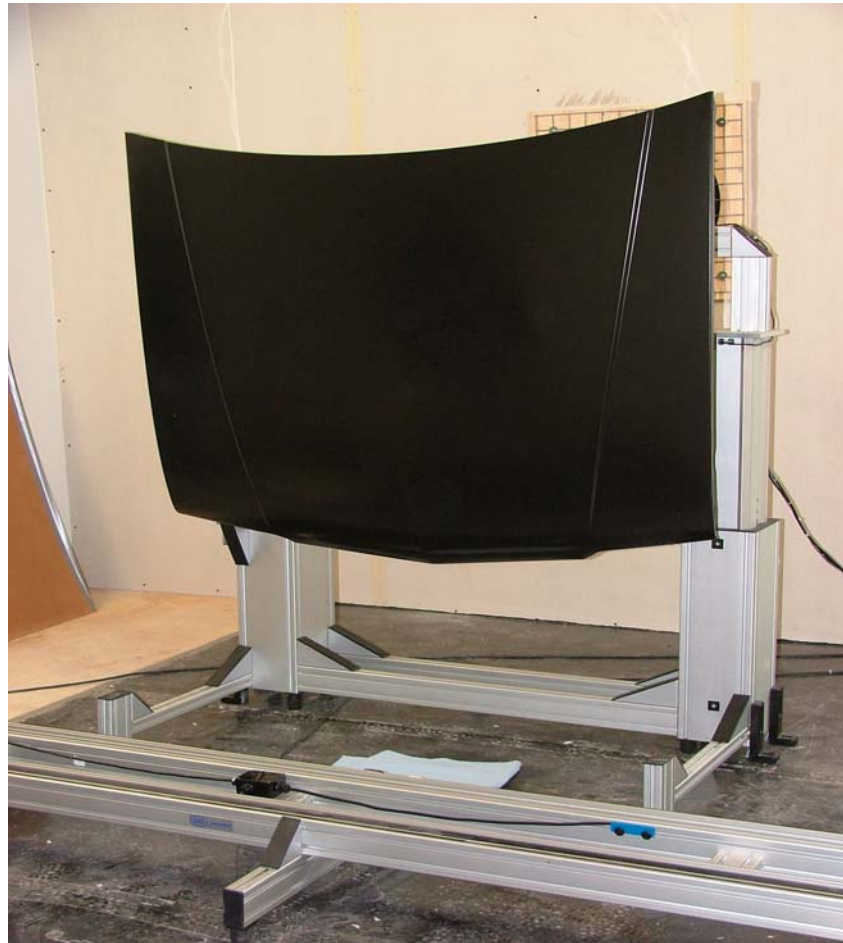
Figure 3. The work piece holding apparatus showing the lifting columns
