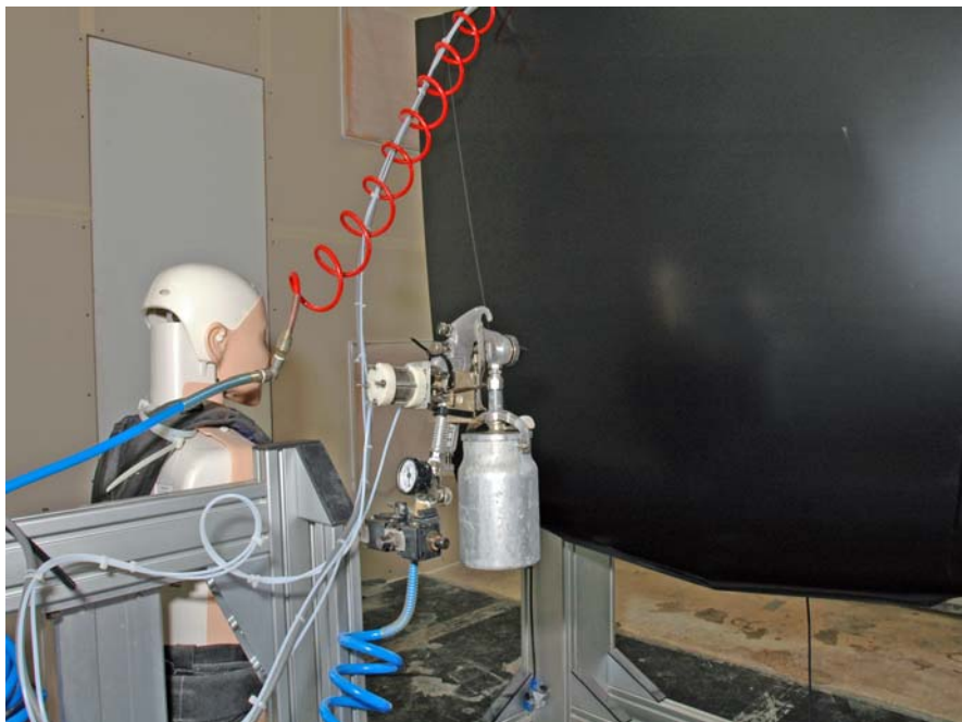
Figure 2. The position of the manikin in relation to the spray gun
