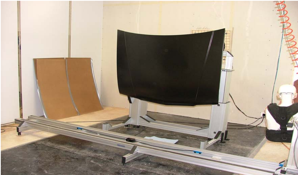
Figure 13. Automatic Sprayer Traversing System– Initial set-up of Spray Room
