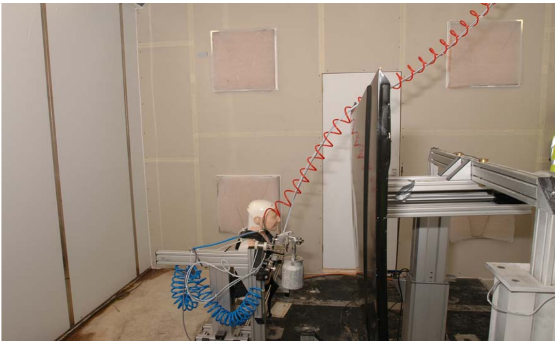
Figure 16. Spray room configuration 2 (Experiments 21 and 22) – note false front wall containing filter panels
