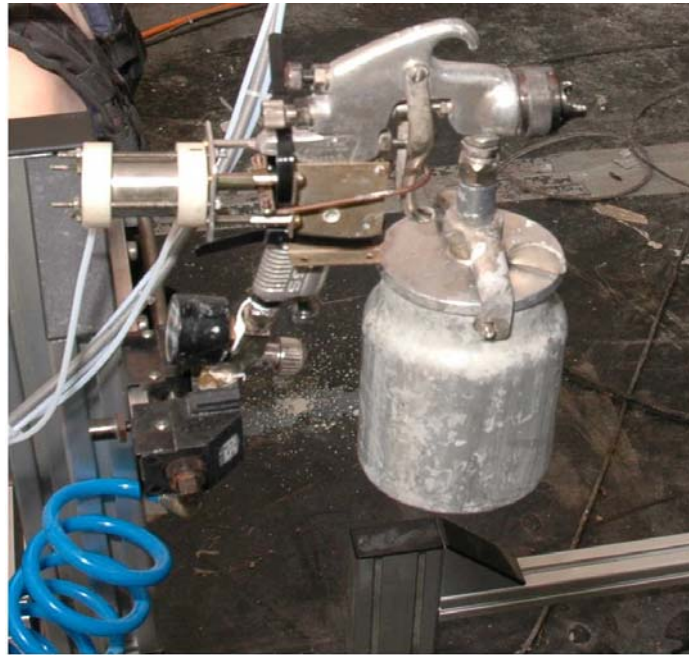
Figure 4. The spray gun and pneumatic actuator
