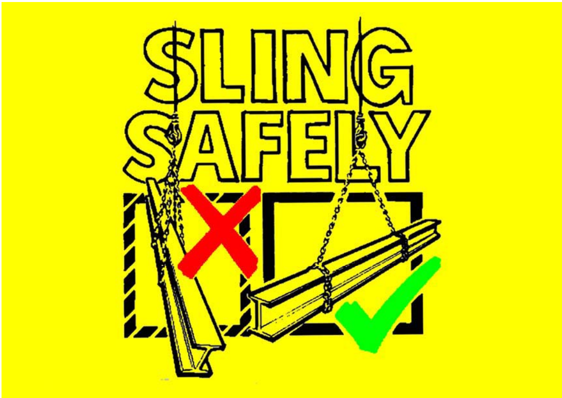
Figure 5 Message used to show right and wrong way of slinging components
