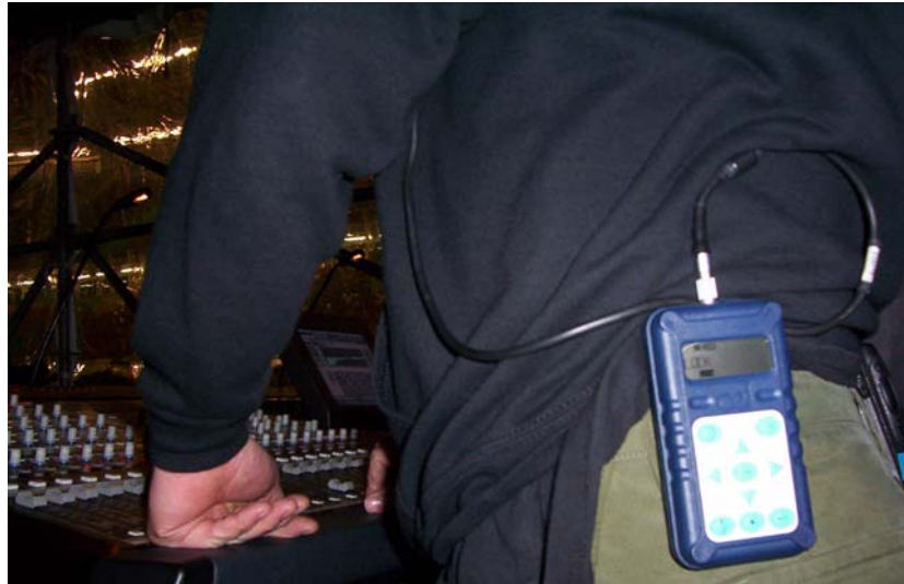
Figure 4.1 - Dosemeter worn by FOH engineer
